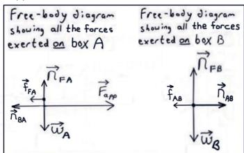
(b) The boxes both have acceleration 2.3 m/s², to the right. Box A exerts a force of 455 N, to the right, on Box B. Box B exerts a force of 455 N, to the left, on Box A.
