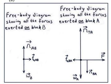
(b) A horizontal force with maximum magnitude F = 63 N can be exerted without the 4 kg block sliding off the 12 kg block.
